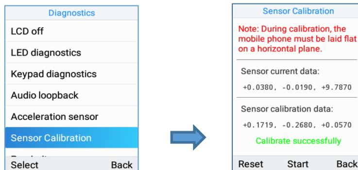
Figure 104: Sensor calibration
